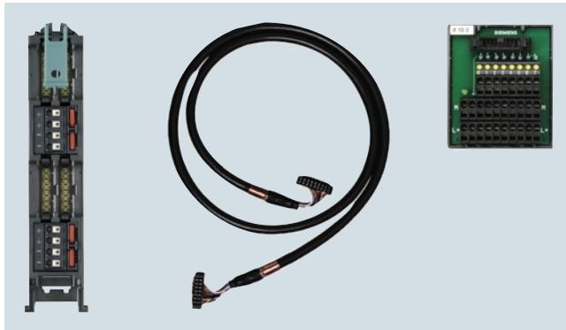
The fully modular connection for connecting to the I/O modules of the SIMATIC S7-1500 or ET 200MP consists of modified front connectors, called front connector modules, preassembled connecting cables of various lengths, and terminal modules. Suitable components can be selected for the application in question and joined by means of simple plug-in connections. The terminal modules are used instead of conventional terminal blocks and act as the interface to the sensors and actuators.
