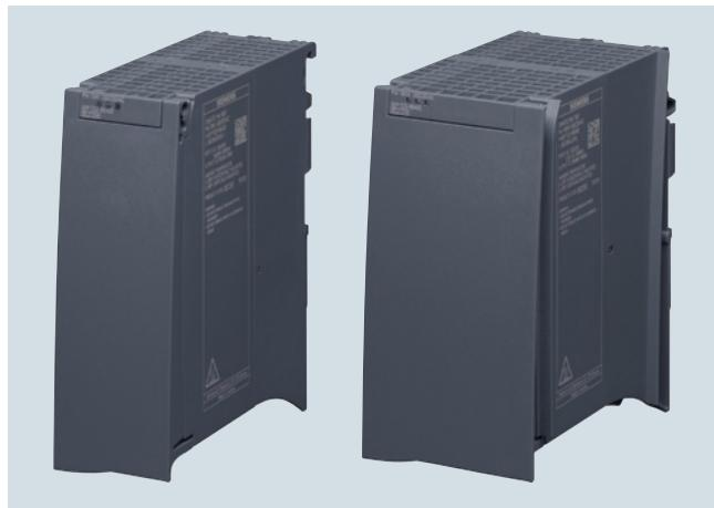
The design and functionality of the SIMATIC PM 1507 single-phase load power supply (PM = power module) with automatic range selection of the input voltage are an optimal match to the SIMATIC S7-1500 PLC. It supplies the S7-1500 system components such as CPU, system power supply (PS), I/O circuits of the input and output modules and, if necessary, the sensors and actuators with 24 V DC.
